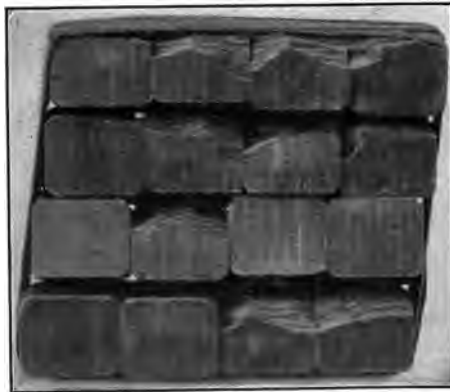
FIG. 85.—Fractured brushes as a result of brush chatter, due to high mica and a rough commutator surface.
